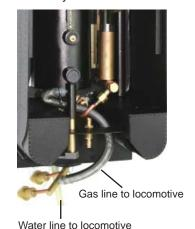
Remove the lubricator cap and draw Firing up out any water from previous run with a syringe. Use only proper steam cylinder oil. Fill the lubricator, but leave a small air space between the oil and the cap.
